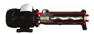
The RL series is an extremely compact product thanks to the integrated pump-electric motor construction. The patented pin joint of the Diamond series ensures high reliability. The support between the body pump and drive unit has been eliminated which makes the pump more compact and easier to maintain.
