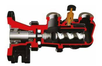
The RF series is based on the same technology as the R series. The difference lies in its use of a bearing unit with plug-in shaft. The RF series can be flanged directly to the drive. This is the ideal solution for the supply of a pump without a drive system, while maintaining compactness and easy installation. The bearings ensure the highest reliability in all operating conditions
